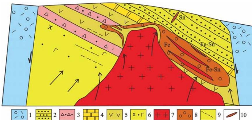
图3 内蒙古黄岗矽卡岩型铁锡矿床模式图<sup>[28]</sup>Fig.3 The model map of the Huanggang skarn iron–tin deposit in Inner Mongolia<sup>[28]</sup>
